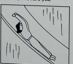
⑤ 手を挙げ足を そろえて降下する Descend in chute with arms stretched upward and legs stretched and contact together.
