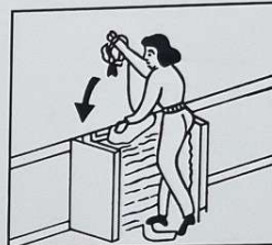
③ 投げ網の 砂袋を投下し Throw down sandbag that guide rope.
